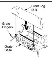
Figure 24 - Installing Front Log (#1) (CCL3930PR/NR Shown)
